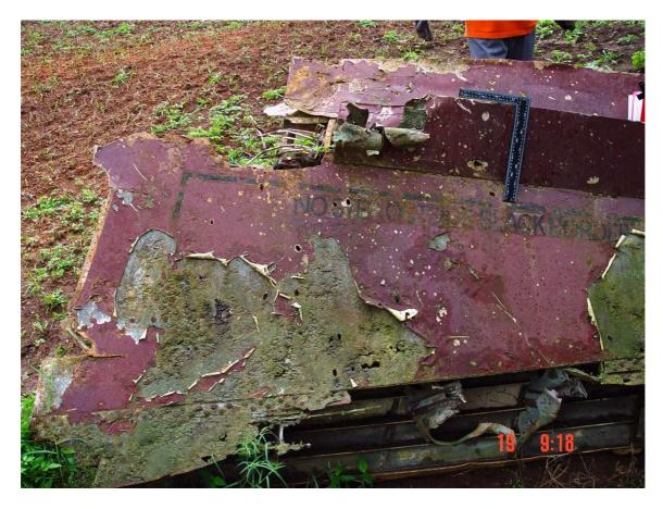
Fig. 22: Rear Section of Left Wing (1).
