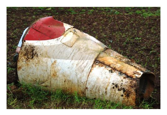
Fig. 20: Tail Exhaust Cone.
